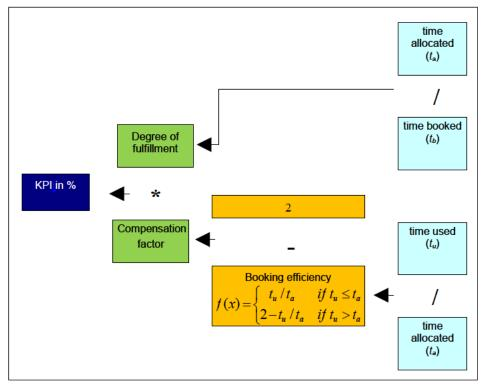
Figure 4: Way of calculating KPI: Performance of the ASM process with regard to request/allocation/use of ARES
